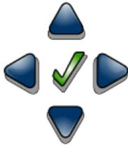
Modifying values through the touch-screen display is accomplished through the use of the data entry panel. The data entry panel provides up, down, left, right and checkmark buttons. Using these buttons, modifications to numeric values can occur in one of two ways: an *up/down method* or an *individual digit method*.
