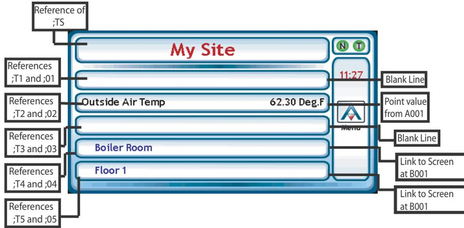
Figure 4-2 Home Screen Configuration on SBC-SD
