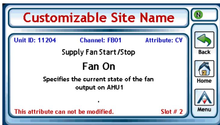
Figure 4-1 Slot Display Information Example
