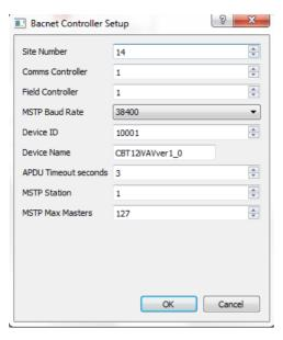
8. From this window the BACnet MS/TP configuration settings can now be configured.
