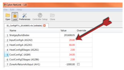
Change the rest of the input and output configuration codes.
