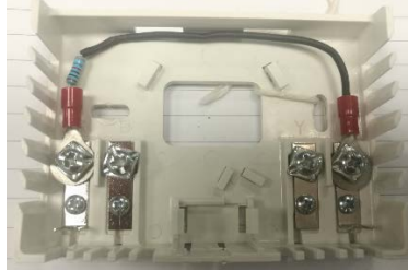
Figure 2: KIT-1RK installed at SBC-STAT
